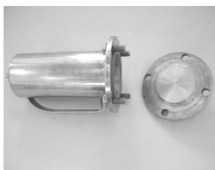
Fig.1. Laboratory autoclave for tretreatment of rice straw
