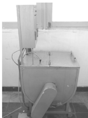
Fig.1. Laboratory autoclave for tretreatment of rice straw
